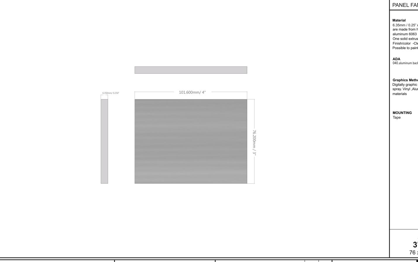
6.35mm / 0.25" Anodized aluminum are made from high quality and recycled
